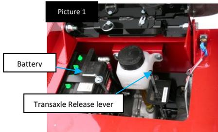
3. Release parking brake if applied. You should be able to roll the machine out of the crate by pushing on the rear bumper. **DO NOT STAND IN FRONT OF THE MACHINE WHILE ROLLING OUT OF CRATE.**
