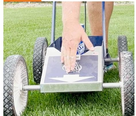
Utilize the arrow on the machine which indicates the center of your spray.
