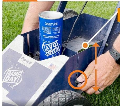
Loosen the adjustment wing nuts to set height of spray. Tighten when done.
