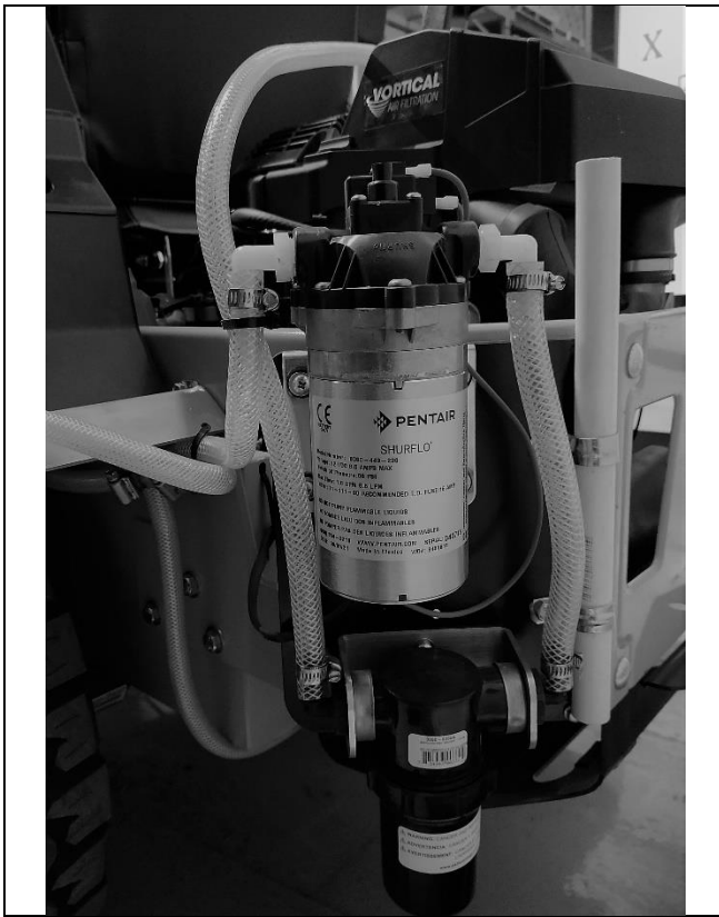
Blitz Tank Pump Connections
