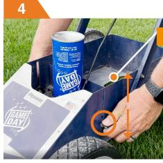
Loosen the adjustment wing nuts to set height of spray. Tighten when done.
