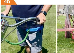
**Method 2:** Release handle on left-side of machine to unlock wheel and maneuver around the circle.
