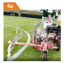
**Method 1:** Lock your front wheel and paint along the outer edge, using the dots as a reference.
