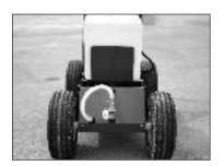
Before striping, make sure the spray nozzle assembly is tight and properly aligned
