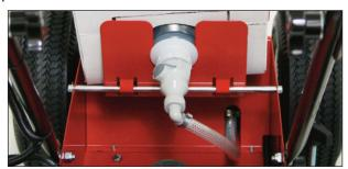
Once secure, lower the StarLine box to the battery cover. You are now ready to begin striping. We recommend practicing in an off area so you can get accustomed to the operation of all switches and to select the tip that best suits your needs.
