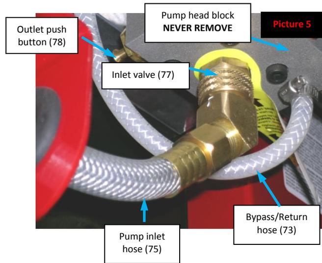
**NEVER REMOVE FRONT COVER, PRESSURE ADJUSTING VALVE, OR THE PUMP HEAD BLOCK.
